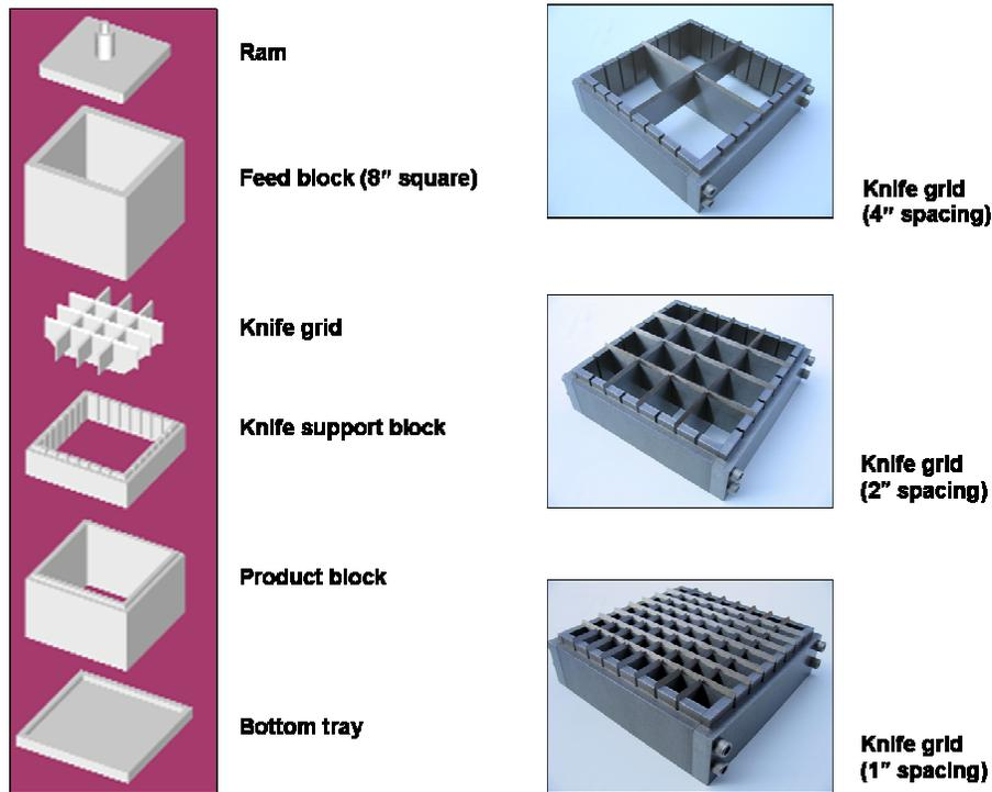
Figure 1. Components of linear knife grid model cutting device and knives arrangement at various grid spacing.
