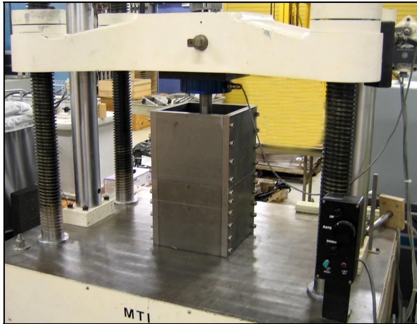
Figure 2. Universal testing machine (MTI; Capacity 22680 kg) with assembled linear knife grid model cutting device being tested.
