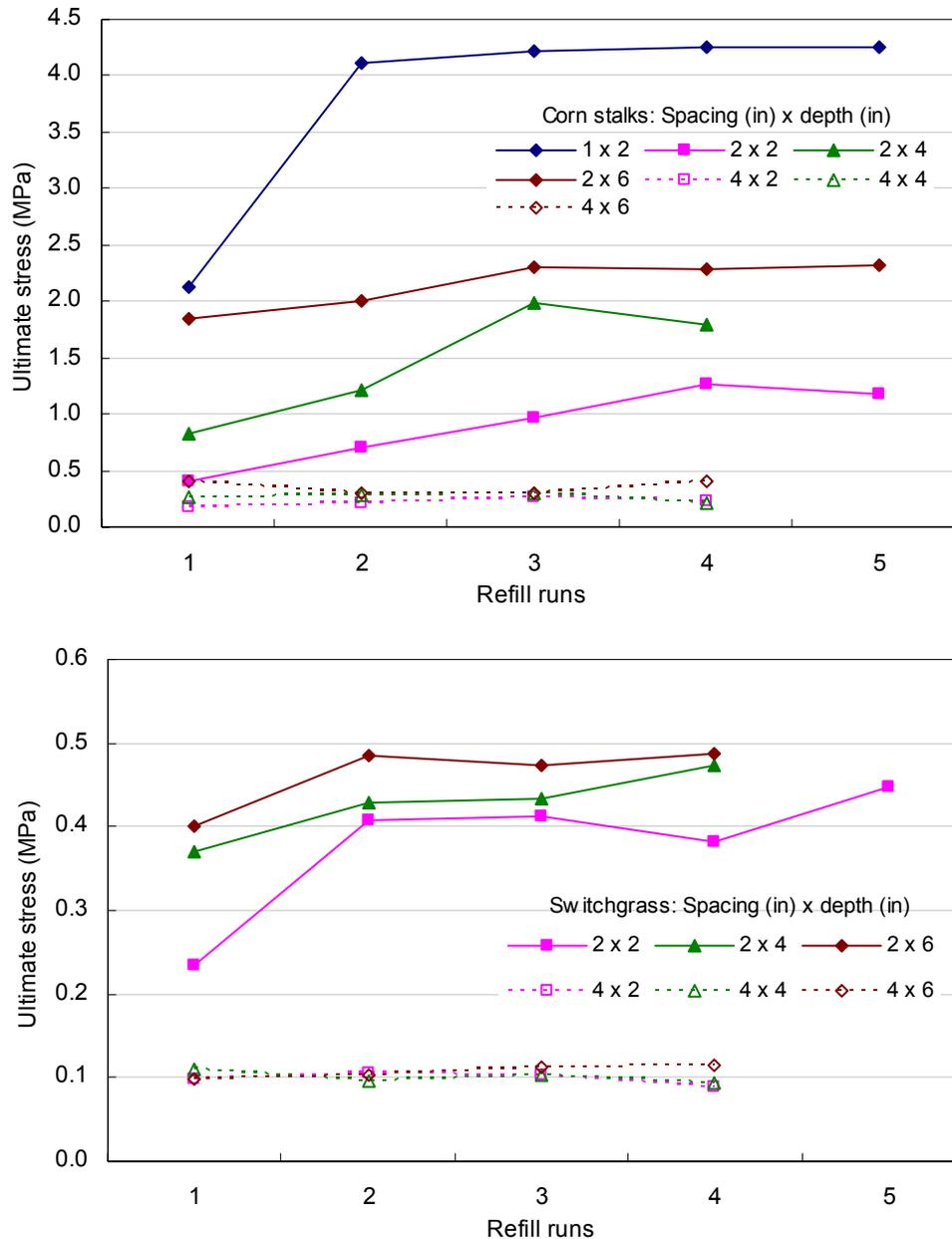
Figure 7. Ultimate cutting stress for corn stalks and switchgrass with different knife grid spacing and fill depths.
