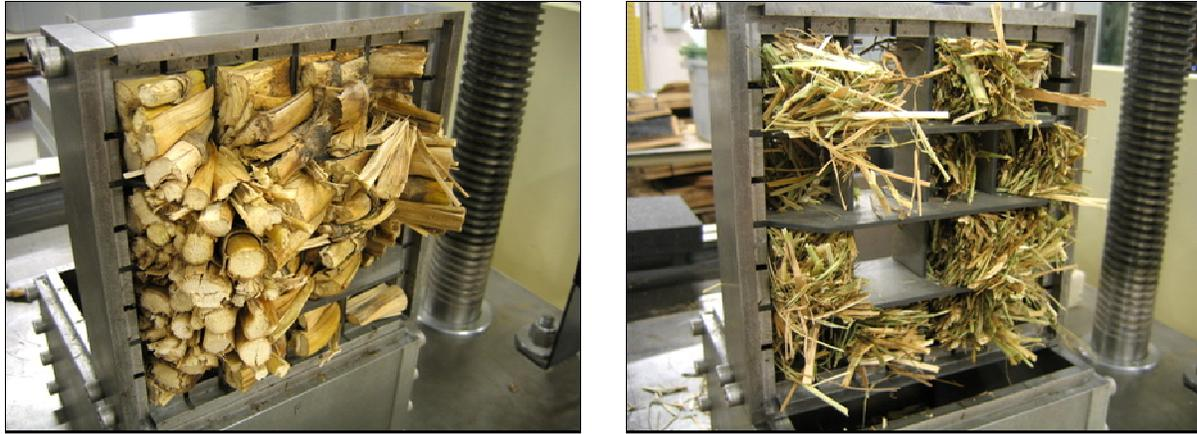
Figure 6. Cut product embedded in the knife grid annular space (50.8 mm (2") knife grid spacing).
