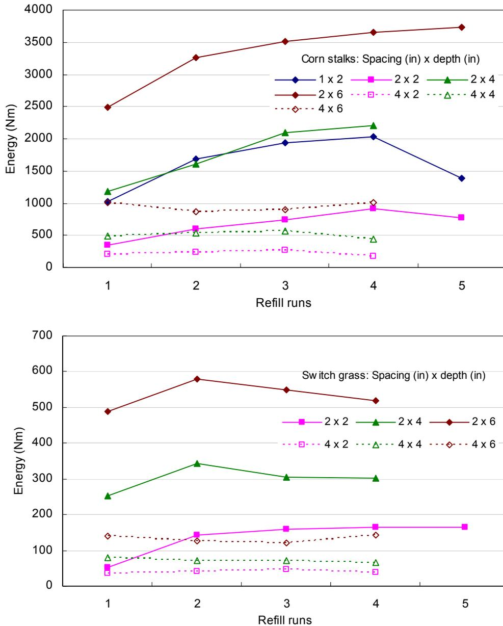
Figure 8. Net energy for corn stalks and switchgrass with different knife grid spacing and fill depths.
