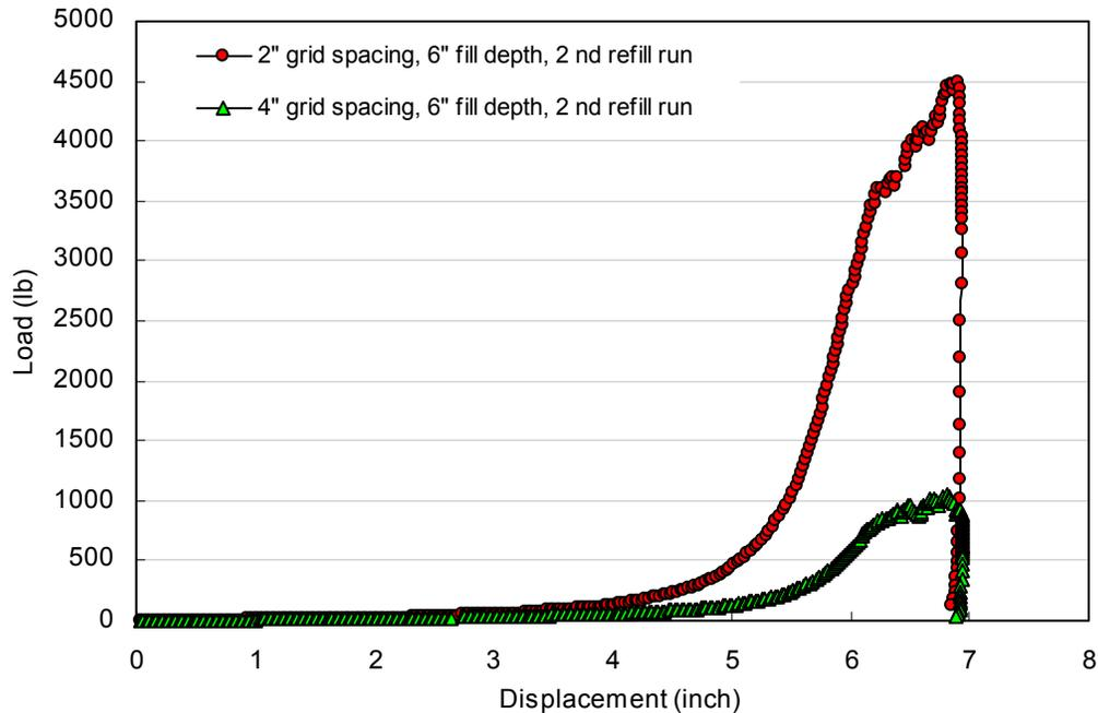
Figure 5. Typical load-displacement cutting characteristics of switchgrass under linear knife grid.
