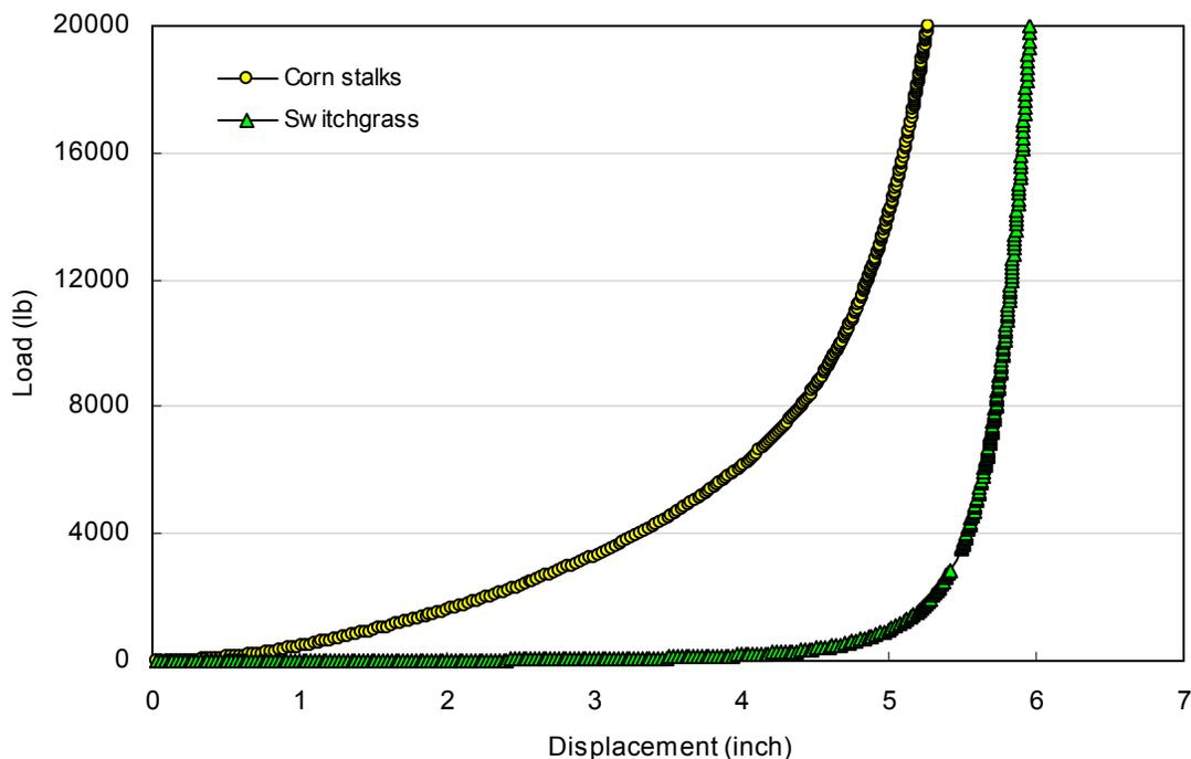
Figure 3. Simple compression characteristics of corn stalks and switchgrass with 6 inch fill.
