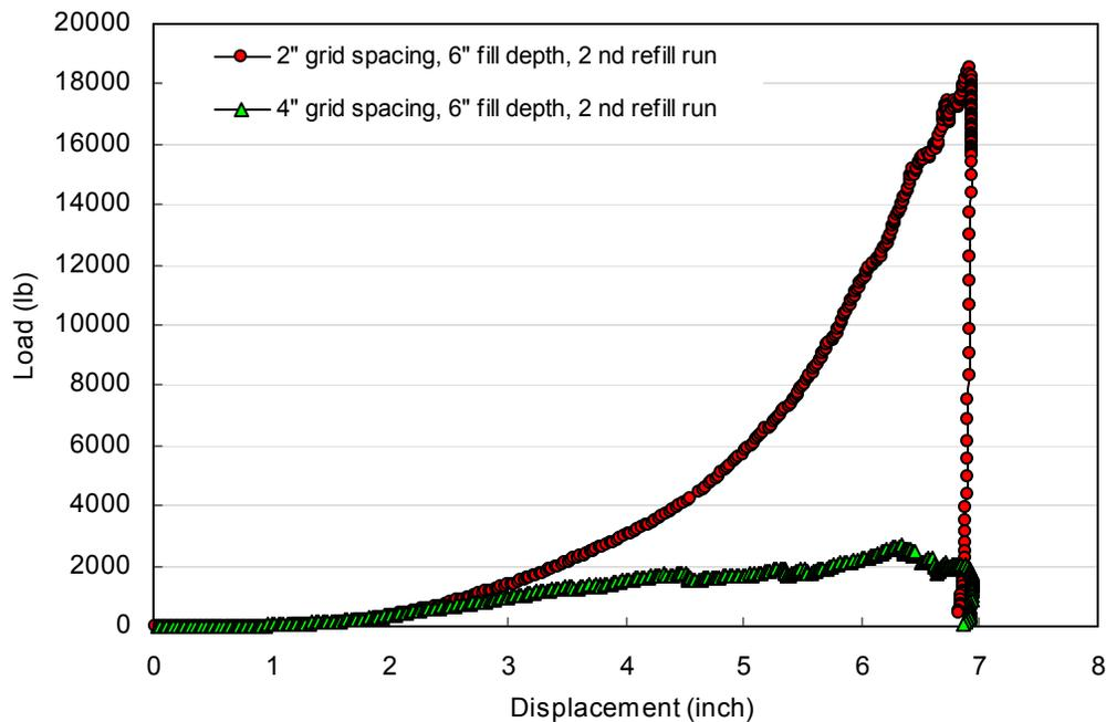
Figure 4. Typical load-displacement cutting characteristics of corn stalks under linear knife grid.
