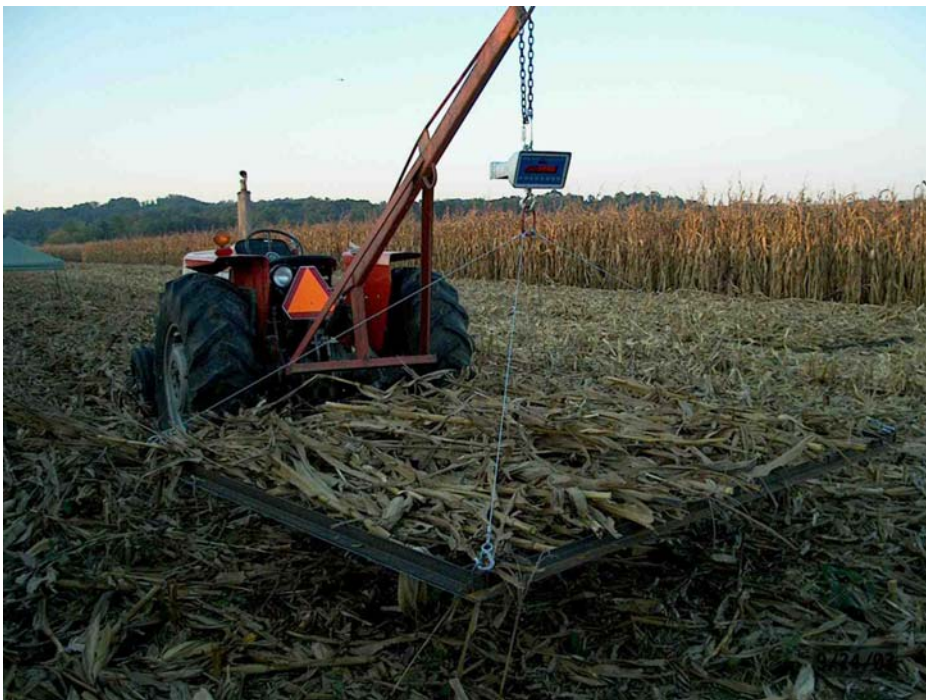
Figure 2. A typical afternoon mass determination of basket loaded with corn stover using a suspended crane scale
